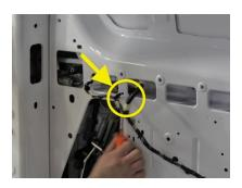
USING A CLAW HAMMER, POP OUT THE PLUG HOLDING THE WIRING HARNESS IN PLACE. AS BEST AS POSSIBLE, TUCK THE WIRING HARNESS INTO THE WALL CAVITY.
