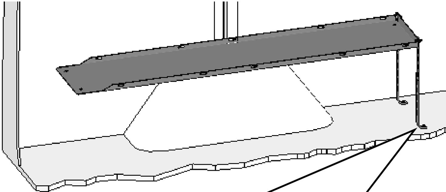
YOU WILL HAVE TO BEND THE SHORT FLANGE OF THE BRACE UP TO 90 DEGREES TO INSTALL AS SHOWN.
