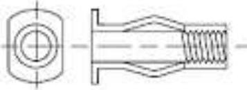
2. The Plusnut is preassembled with a hex cap and hex bolt. Then it is inserted into a predrilled hole.
