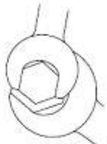
5. A fully upset Plusnut provides a reliable nut for fastening.
