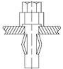
4. The C-500 Plusnut tool tightens bolt through hex head cap into Plusnut. A ratchet, open-end or closed-end wrench can be used.
