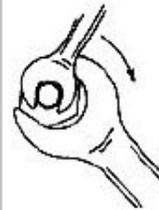
C-500 tool tightens bolt thru hex head cap into Plusnut® A
