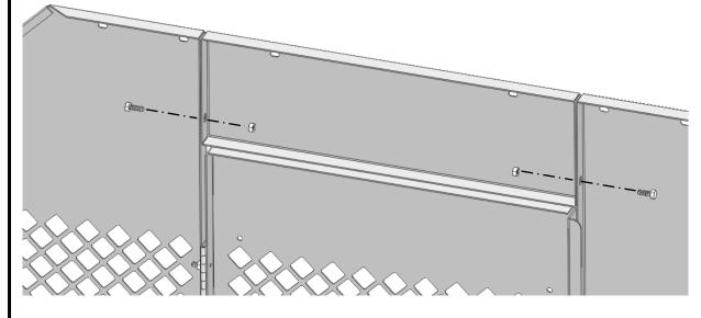
Align holes in Panel as shown and secure using:
