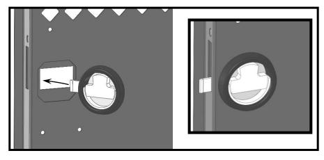
Insert the Round Handle into door cutout, so that the locking mechanism fits through the slot in the Center Panel. **NOTE: Be sure the Locking Mechanism** is parallel to the floor before attaching the inside Handle.
