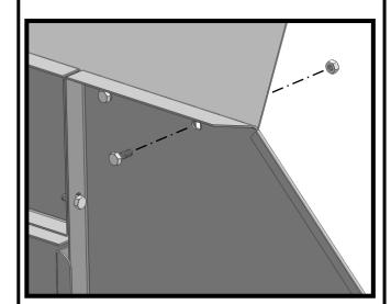
Align holes in Top Panel as shown and secure using:
