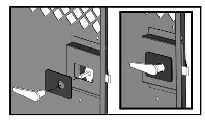
Attach the Plastic Latch Cover Plate and the Chrome inside Handle firmly to the back of the Round Handle. Be sure the inside handle is parallel to the floor, but facing the opposite direction of the locking mechanism.
