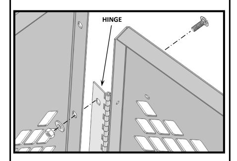
Align holes in Hinge on Door as shown and secure using:
