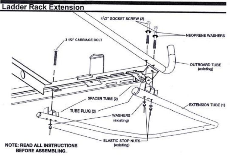
STEP 1: If the Ladder Rack is assembled, remove the socket head screws at the front of the outboard tube and the carriage bolt at the front of the inner rail on the side the extension is to be mounted. Retain the elastic stop nuts, flat washers and neoprene washers for reinstallation.
