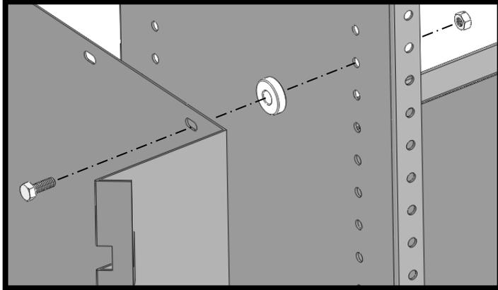
Align holes in Spool Carrier with holes along right hand side of Upright and secure using:
