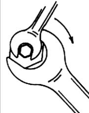
C-500 tool tightens bolt thru hex head cap into Plusnut® A
