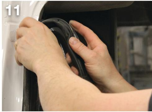
When properly positioned, tighten all bolts. Adjust the weatherstripping along the door frames. The rubber should cover the outer edge of the panel.
