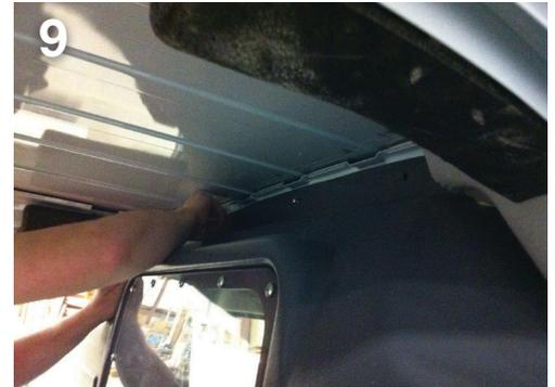
9 Loosely secure the floor and ceiling with the 1 1/2" screws (D), washers (C), and split washers (B).
