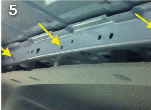
5 Using the three holes at the top of the partition and mark the holes on the pillar. Remove the partition.
