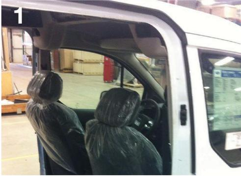
1 Pull back the rubber trim from around the sliding door frames.
