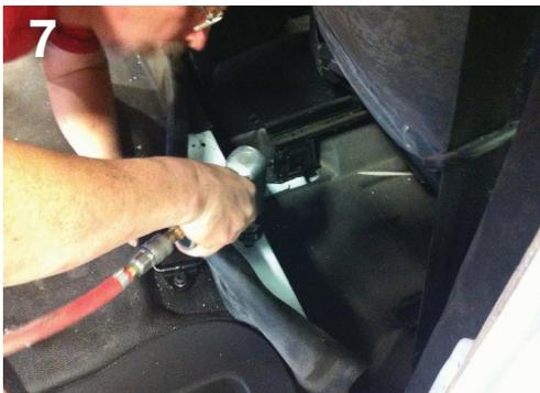
7 Peel back the flooring to reveal the metal underneath. Insert and secure plus nuts (A) using the plus nut gun for the four holes. Place the spacers (F) over the plus nuts before putting the flooring back in place.
