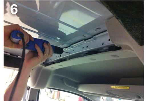
6 Drill pilot holes through each marked hole, then re-drill them using a 11/32" bit. You will be drilling through the van floor.
