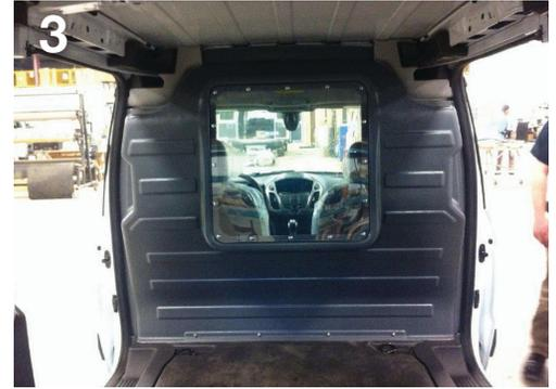
3 Slide the partition into place so that it lines up against the B-Pillar and along the headliner.
