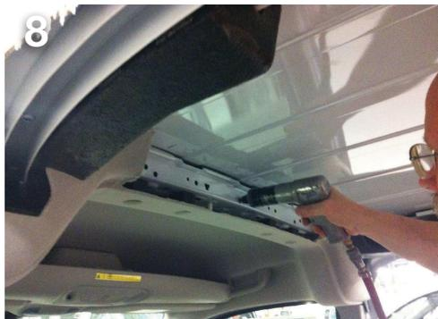
8 Install plus nuts (A) in the three holes in the ceiling pillar with the plus nut gun. Slide the partition into place, aligning the pre-drilled holes to the holes just drilled.
