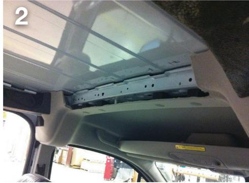
2 Using a knife, trim the headliner along the lower trim line between the inside edges of the outermost ceiling ribs.
